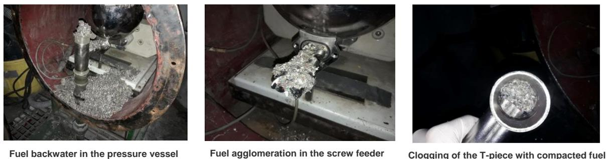
Figure 6. SBS-2 agglomeration in the pressure vessel (left), screw feeder (middle) and T-piece (right).
