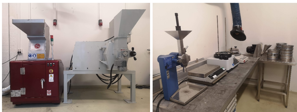
Figure 5 Fuel preparation facility showing the tabletop equipment for milling and sieving to the left and the large-scale mill and pellet-press machine to the right
