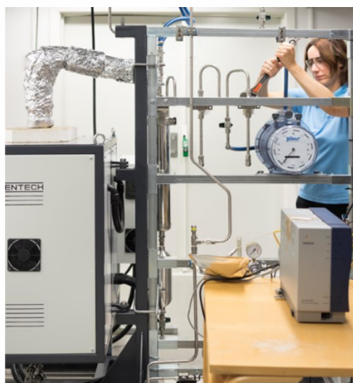
Figure 1 The Pyrolysis and Carbonisation reactor
