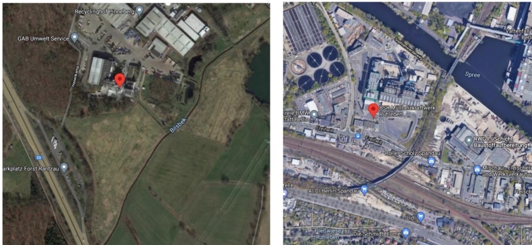
Figure 9: Examples of a WtE plant with no space limitation for CO 2 capture retrofit (AVG KG Tornesch plant in Germany, left) and a plant with insufficient space for retrofit (Berlin City Cleaning WtE plant, right)
