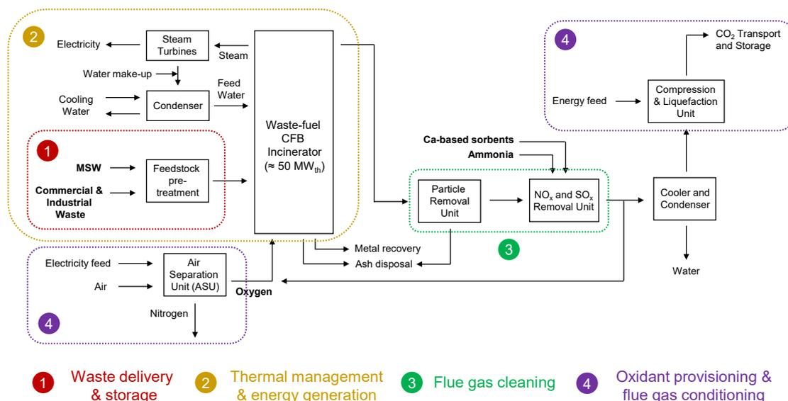
Figure 4 Block flow diagram of the reference oxy-fuel WtE plant with a CFB boiler (Joseba Moreno, 2022)
