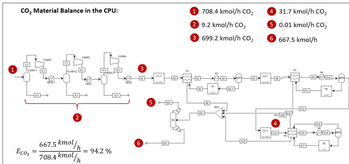
Figure 14 CO<sub>2</sub> Material Balance in the CPU of the Oxy-fuel CO<sub>2</sub> capture facility
