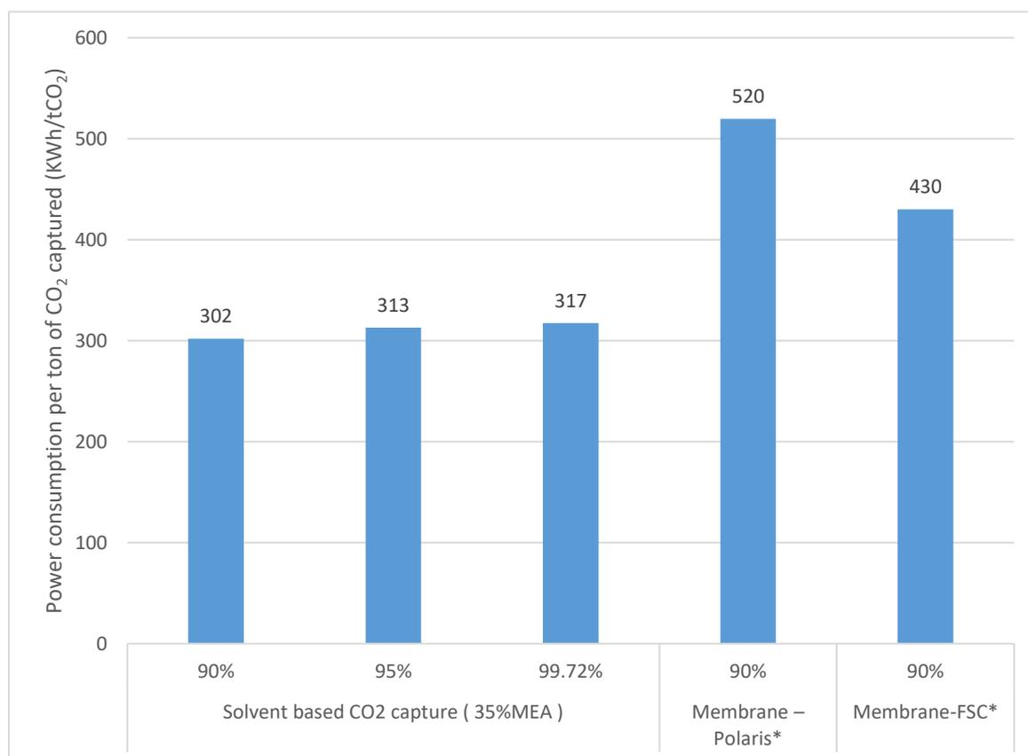
Figure 5 Comparison of the specific power consumption per ton of CO<sub>2</sub> captured for Membrane and MEA cases. Note: For MEA cases, the specific power consumption per ton of CO<sub>2</sub> captured is using electricity output penalty per ton of CO<sub>2</sub> captured, which is the difference of power output before and after CO<sub>2</sub> capture.
