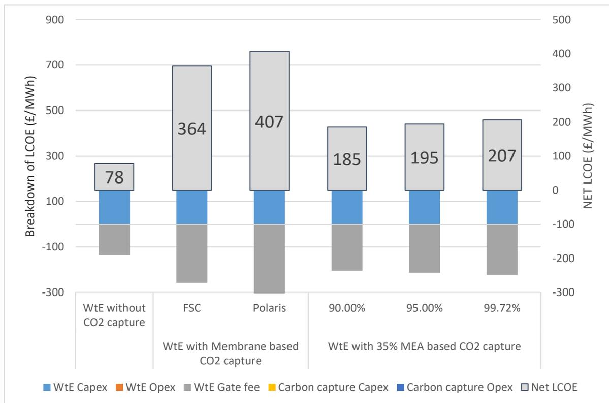
Figure 6 Breakdown of LCOE of WtE plant under Membrane cases 90% capture (FSC and Polaris) and 35% MEA cases for three CO2 capture rates (90%/95%/99.72%)
