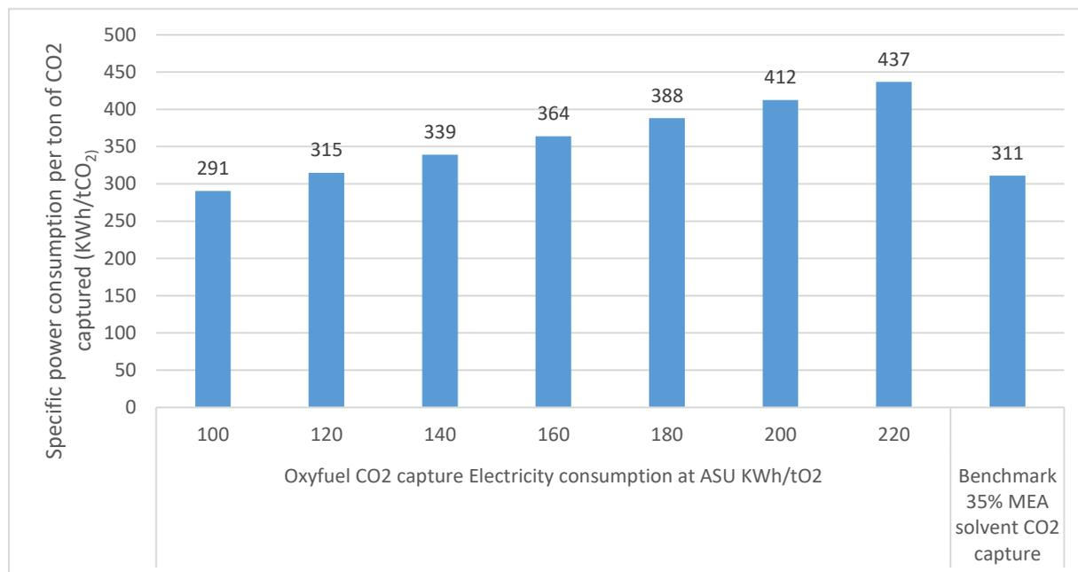
Figure 13 Specific energy consumption for Oxy-fuel CO<sub>2</sub> capture and Benchmark 35% MEA solvent CO<sub>2</sub> capture
