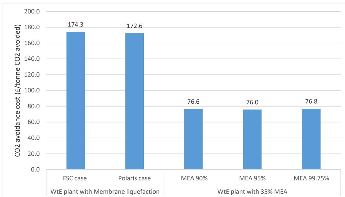
Figure 8 Comparison of CO<sub>2</sub> avoidance cost for Membrane cases at 90% capture rate (FSC, Polaris) and 35% MEA cases at 90%, 95% and 99.72% capture rates.
